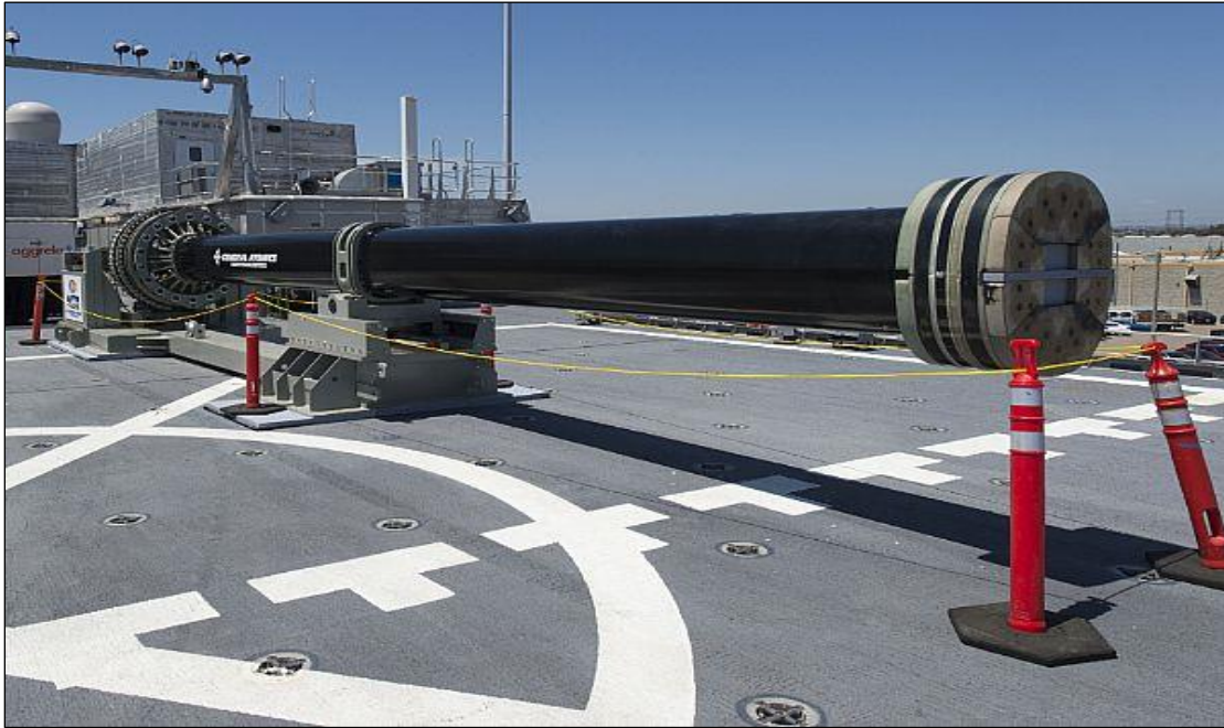
Figure 8. Industry-Built EMRG Prototype Demonstrator General Atomics prototype
