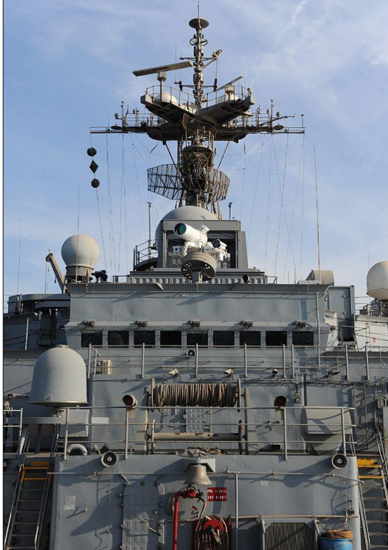
Figure 3. Laser Weapon System (LaWS) on USS Ponce
