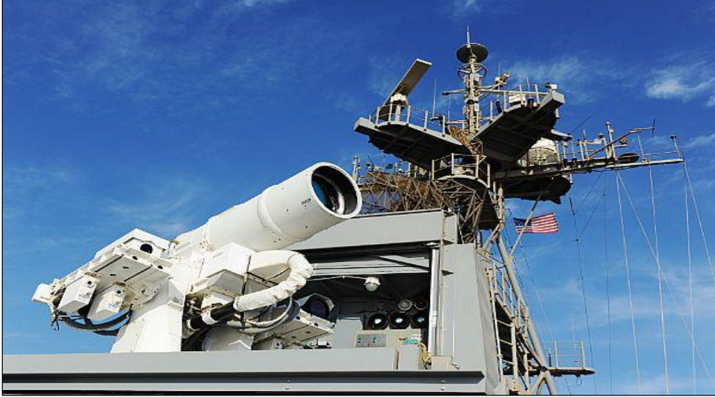
Figure 1. Laser Weapon System (LaWS) on USS Ponce
