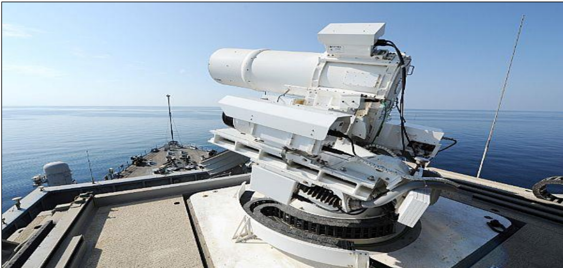
Figure 2. Laser Weapon System (LaWS) on USS Ponce
