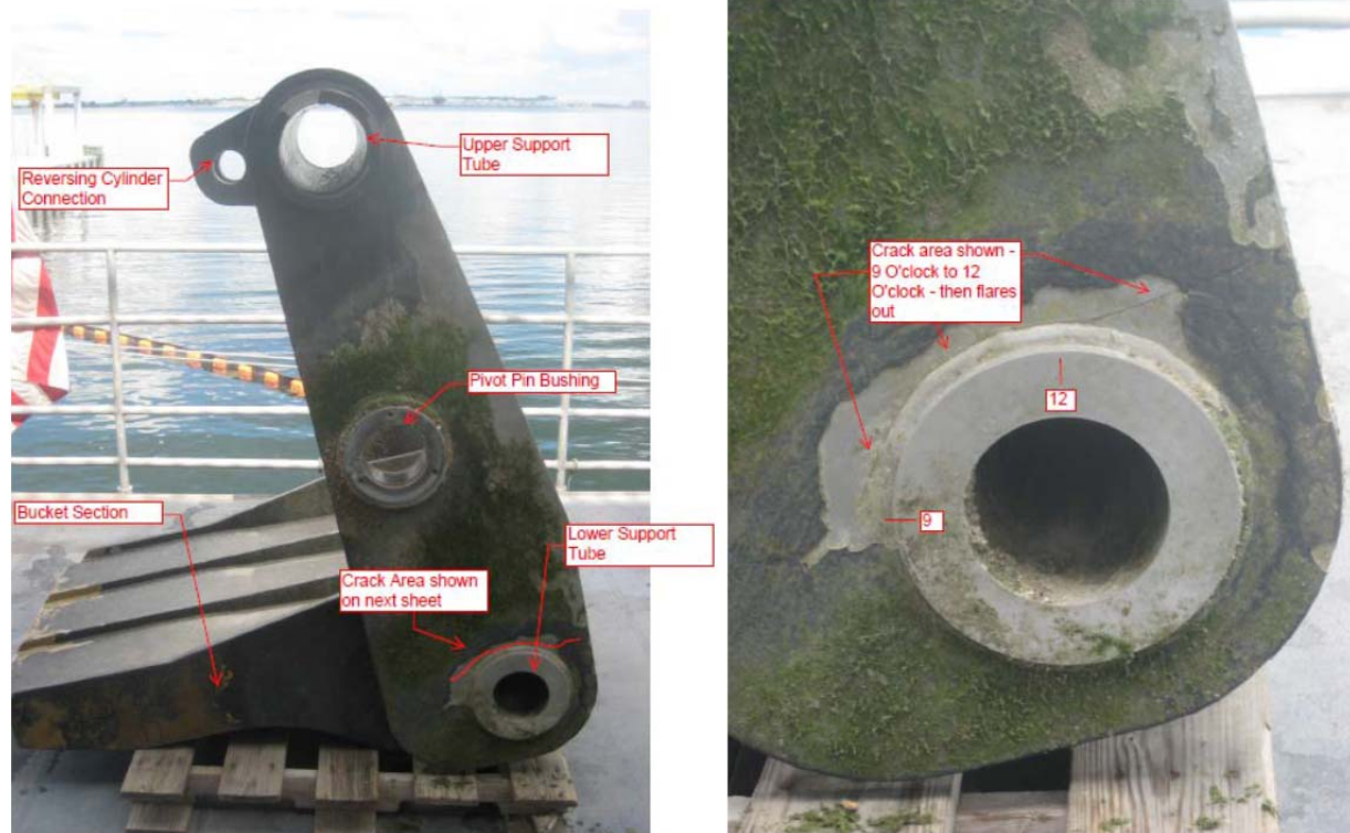
Figure 14. USNS Spearhead Port Waterjet Reversing Plate showing Fatigue Crack
