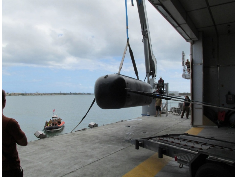
Figure 5. SDV Suspended While Trailer is Removed
