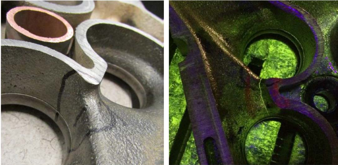
Figure 11. Section Cylinder Head Showing Crack of internal Port
