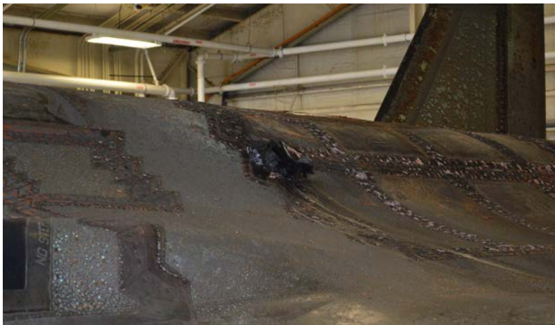
Fig-11. Hole in top of aircraft (Tab S-5)
