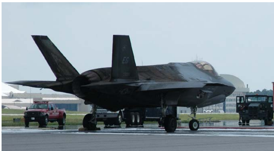
Fig-23. Fire damage post mishap (Tab S-2)
