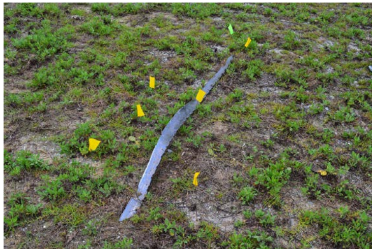
Fig-13. Fragment of R3 forward integral arm (Tab S-3)
